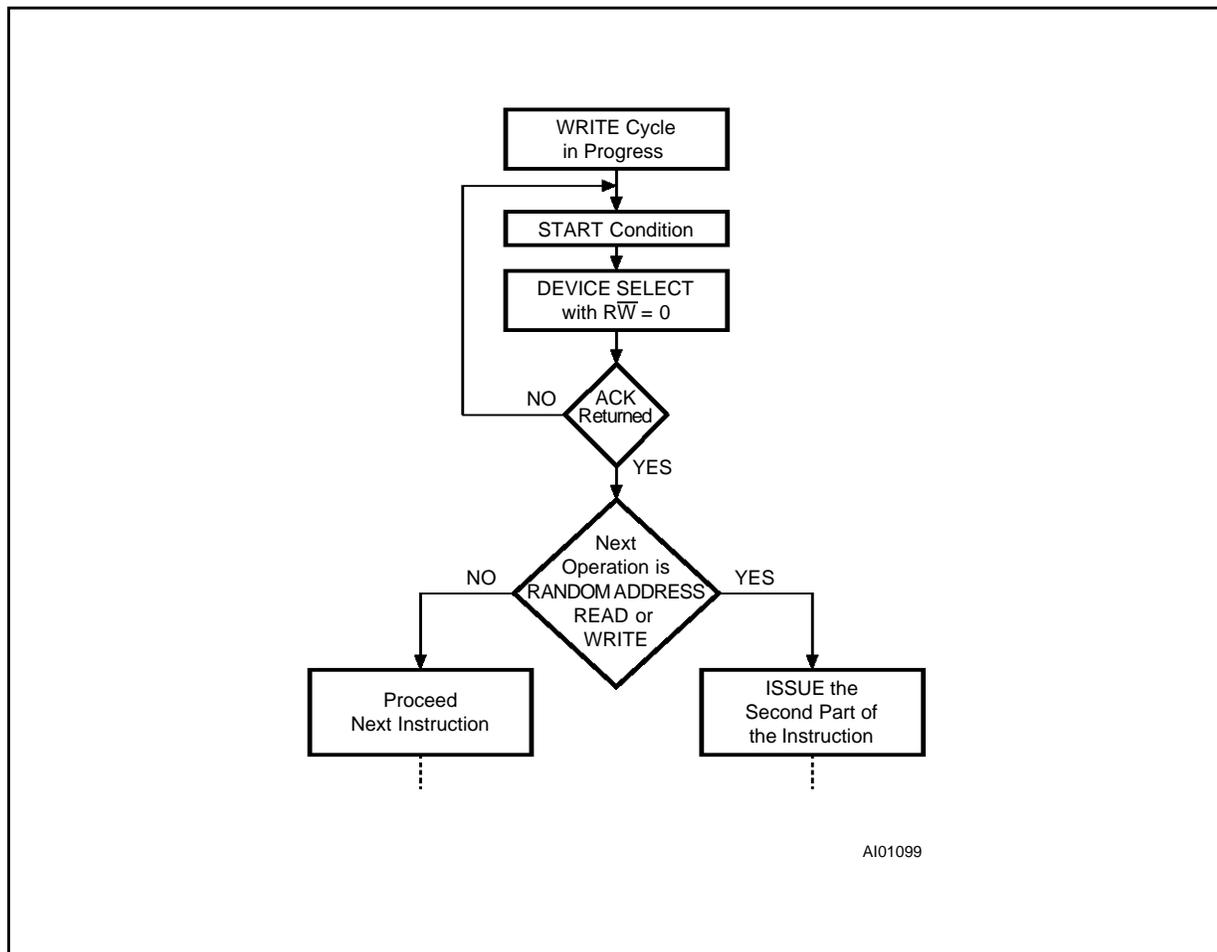
Figure 8. Write Modes Sequence with Write Control = 0
